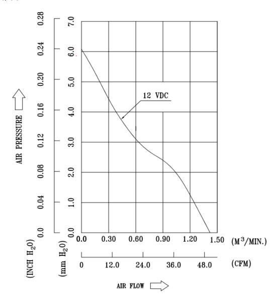
\*TEST CONDITION: INPUT VOLTAGE-----OPERATION VOLTAGE
