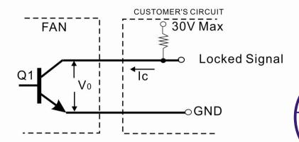
\*Transistor Q1 at "ON" position
