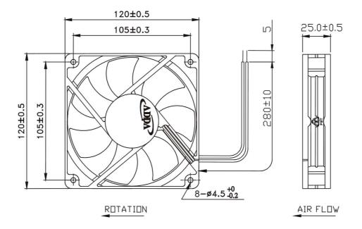
LEAD WIRES: UL 1007, AWG24; L =280±10 mm Red = positive; Black = negative.
