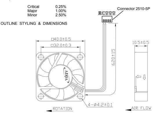
LEAD WIRES : UL 1007, AWG26  $\,$  2510-5P  $\,$  , L = 620  $\pm$  15 mm Red = positive; Black = negative.
